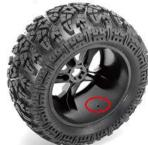
▶ If you feel driving in water is necessary, please seal all holes in the tires and rims before performing this action to prevent the tire foam from absorbing water inside the tires.
